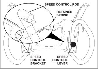
INSTALL TRACTION DRIVE CONTROL ROD (See Figs. 3 and 4)
